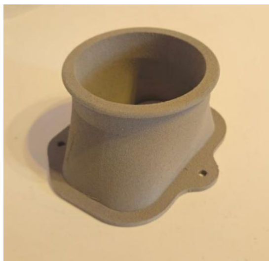
Figure 8. "Grill Intake Adapter" part, manufactured using PLA filament on Creality K1C
