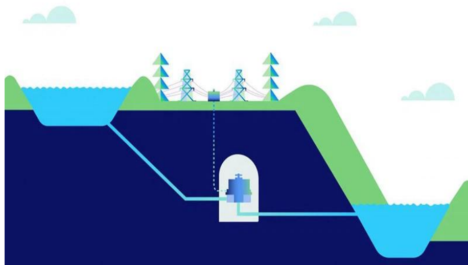
Fig. 1. Hydro power plant with pumping accumulation – the operating principle
