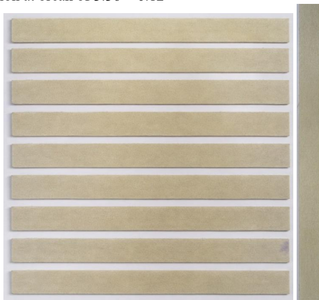
Fig. 1. Samples used for the tensile test (50:50 ratio)
