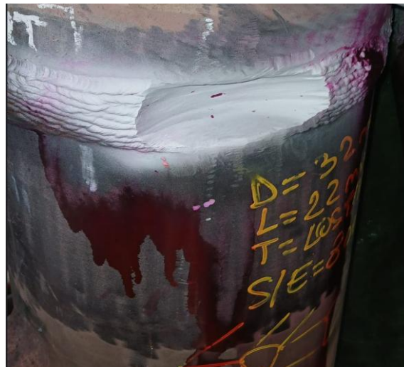
Figure 8. Penetrant testing examination
