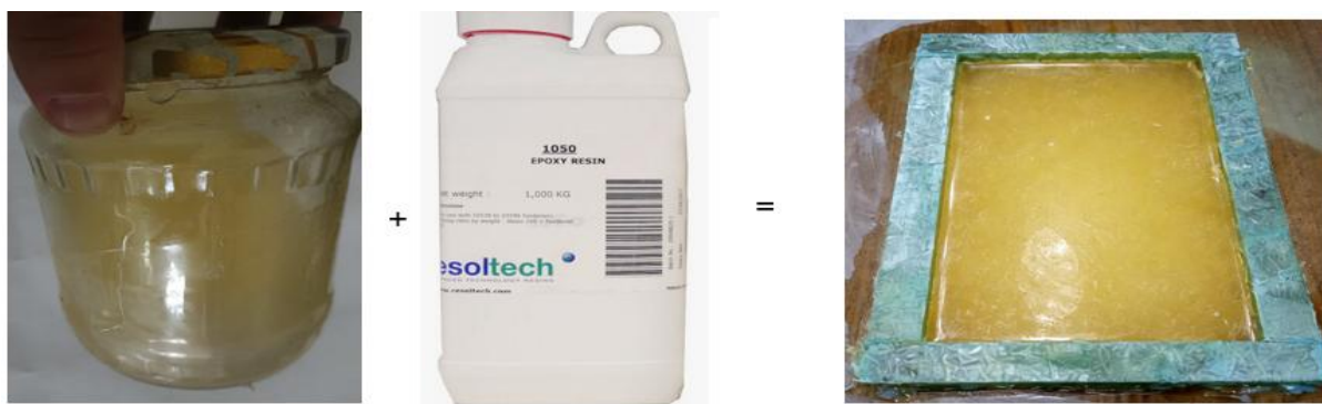
Fig. 2. Schematic representation of the preparation of a bio-based dammar-epoxy resin in a 50:50 ratio
