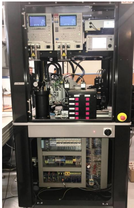
Fig. 2. – Constructive structure of the system: rotary table, electrical cabinet and process subsystems.
