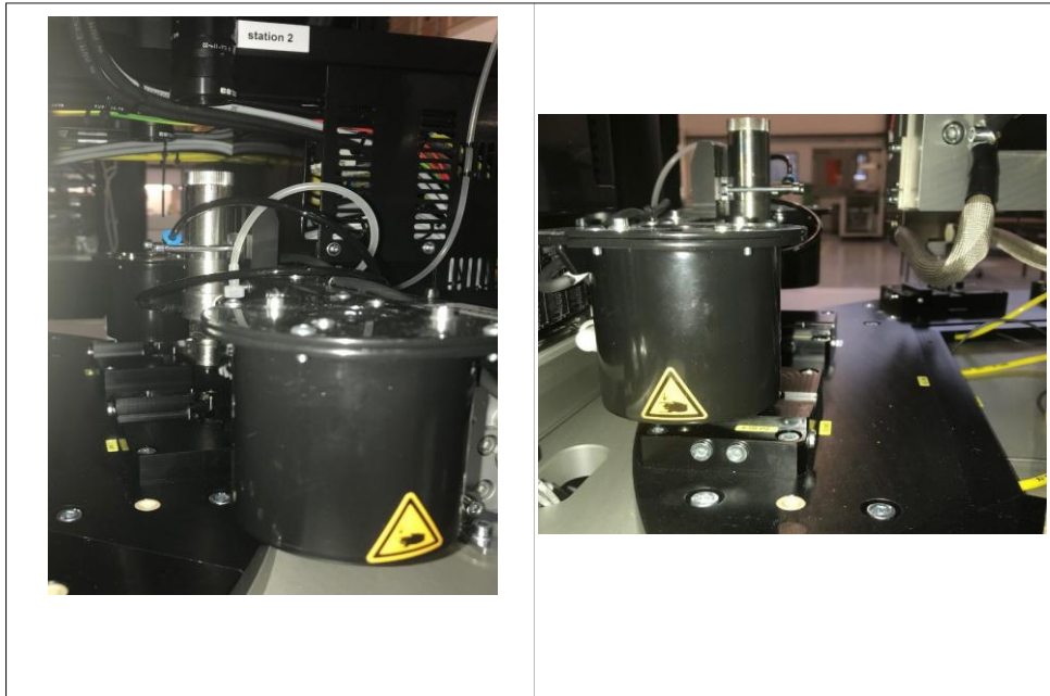
Fig. 5 – Application of the flow and verification of the degree of coverage using industrial vision system.
