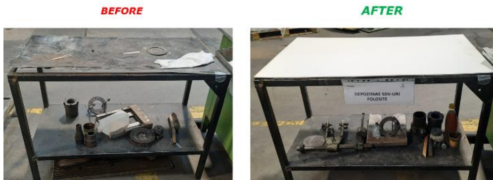
Figure 7. Application of 2S – devices
