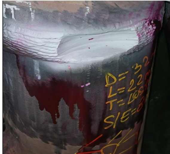
Figure 8. Penetrant testing examination
